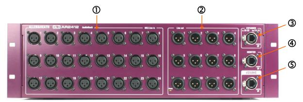
Input sockets 24 balanced XLR inputs for microphone and line level sources. The preamps are built into the AR2412 rack and their Gain, Pad and 48V phantom power is remote controlled from the mixer via the dSNAKE link. The output of the analogue preamps are converted to digital format and transported via dSNAKE to be processed and mixed at the GLD or Qu mixer.
