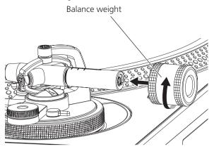
When using a cartridge between 9.5 g and 13 g, attach the sub weight on the rear shaft of the tone arm.
