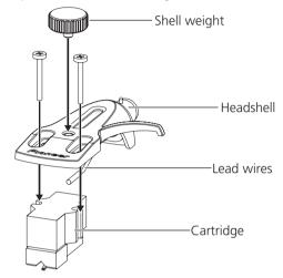
When using a cartridge between 3.5 g and 6.5 g, use the supplied shell weight.
